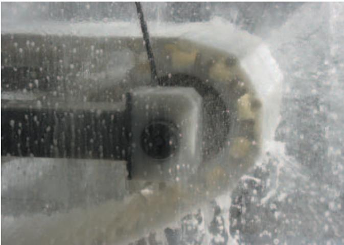
The ModulCLEAN System is installed by replacing an idler roller with a ModulCLEAN unit, and connect the water supply. A detergent/sanitizer supply can also be connected, if desired.
